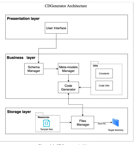
Figure 4-1. CDGenerator Architecture.
